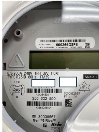
Figure 1: Example of new smart meter with internal disconnect
