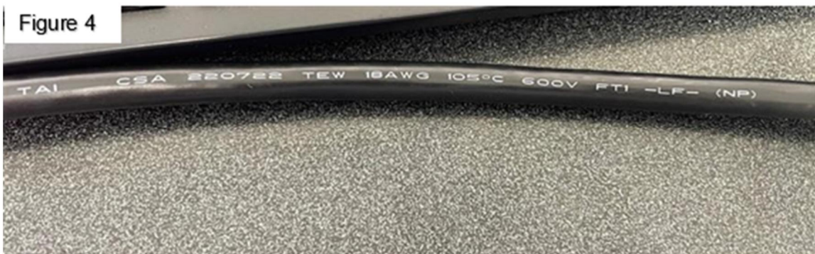
Figure 4: Noncompliant cable (no SJTOW marking)
