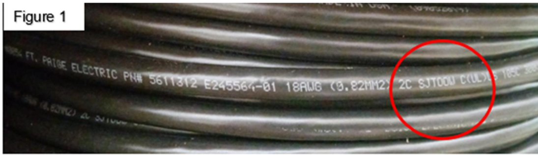
Figure 1: Compliant cable (SJTOW marking)
