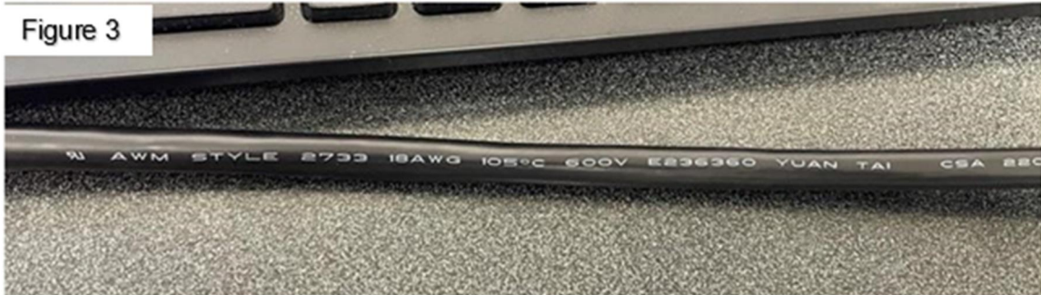
Figure 3: Noncompliant cable (no SJTOW marking)
