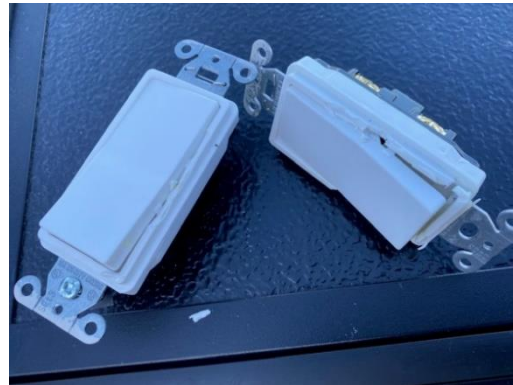
Picture 2, Deterioration Damage to Switch
