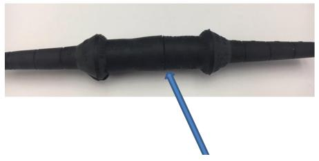
When properly mated, the seam between housings should not exceed 1/32 inch as outlined in the manufacturer's instructions
