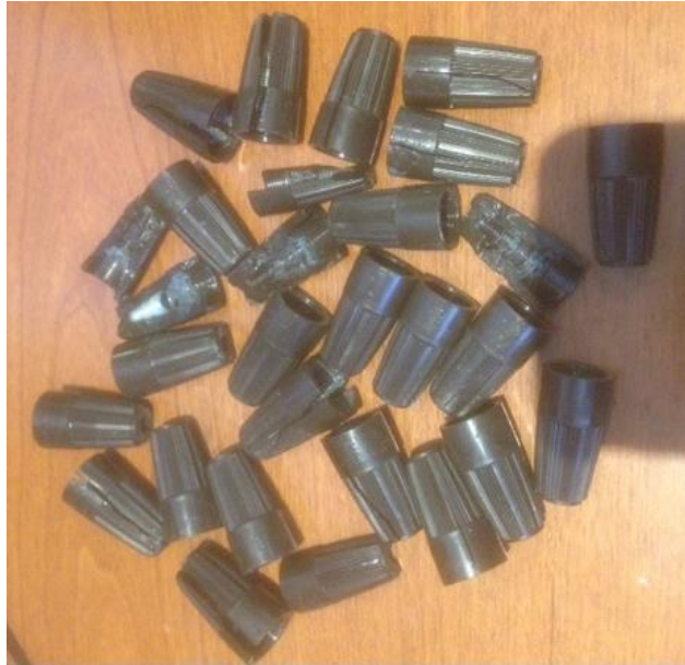
Photo F3 – Non-Petroleum based inhibitor failures
