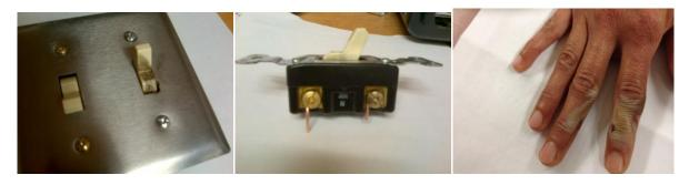
Other switching devices such as relays, contactors and switch rated circuit breakers may also be affected. Manually operated switches are a particular concern, since the user's hands are in contact with the device. Excessive inrush current can cause switch contacts to wear prematurely and, in some cases, arcing across the switch contacts can cause an arc to be emitted.
