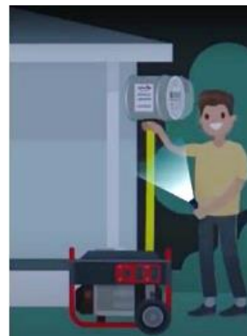
Diagram B1 - Meter-mounted transfer switch plug-in generator
