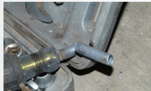
Figure 2. Damaged nut driver after arc flash event.
