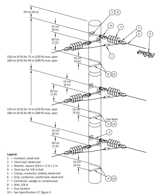
Note: Guy under centre phase not required if conductors utilized are 1/0 AWG or smaller.
