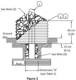
Installation for poor soil
