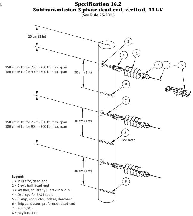
**Note:** *Guy under centre phase not required if conductors utilized are 1/0 AWG or smaller.*
