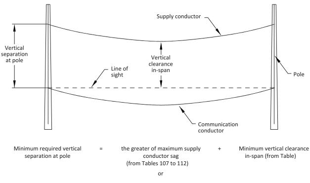
Minimum vertical separation at pole (from Table)
