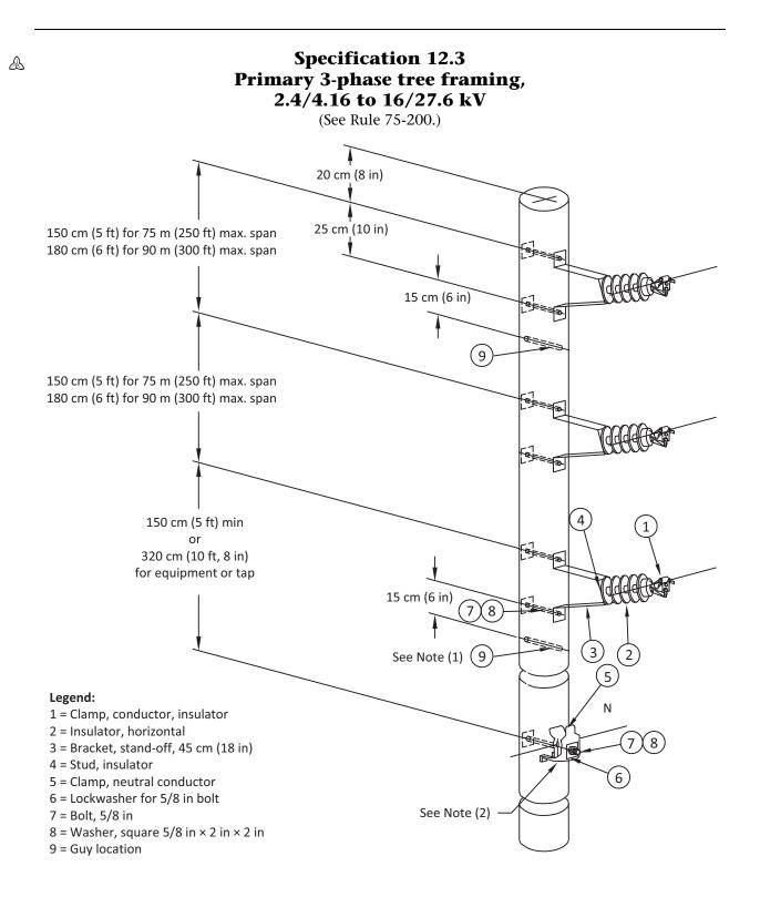
(1) Guy at lowest level phase not required if conductors utilized are 1/0 AWG or smaller.
