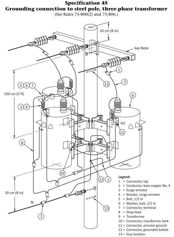
**Note:** Rule 75-804 requires steel crossarms to be connected to a ground electrode where porcelain dead-end insulators are used with a copper conductor.
