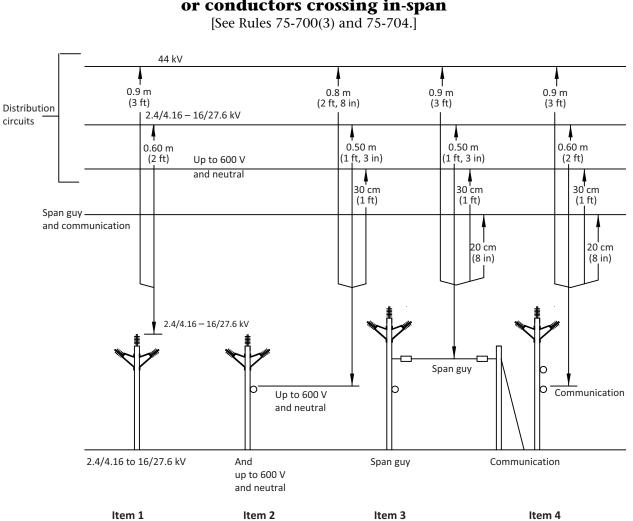
Specification 1 Minimum vertical clearances between wires or conductors crossing in-span
