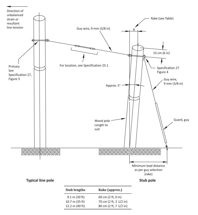
Note: If stub pole carries power circuit, refer to Specification 3, excluding pole offset requirements.
